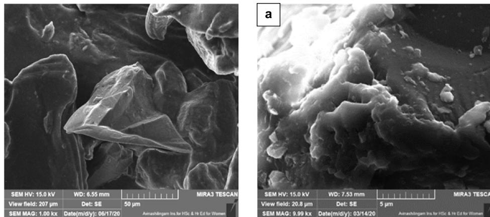
Fig. 3. FESEM micrographs of (a) raw adsorbent and (b) seafood processing effluent treated adsorbent
