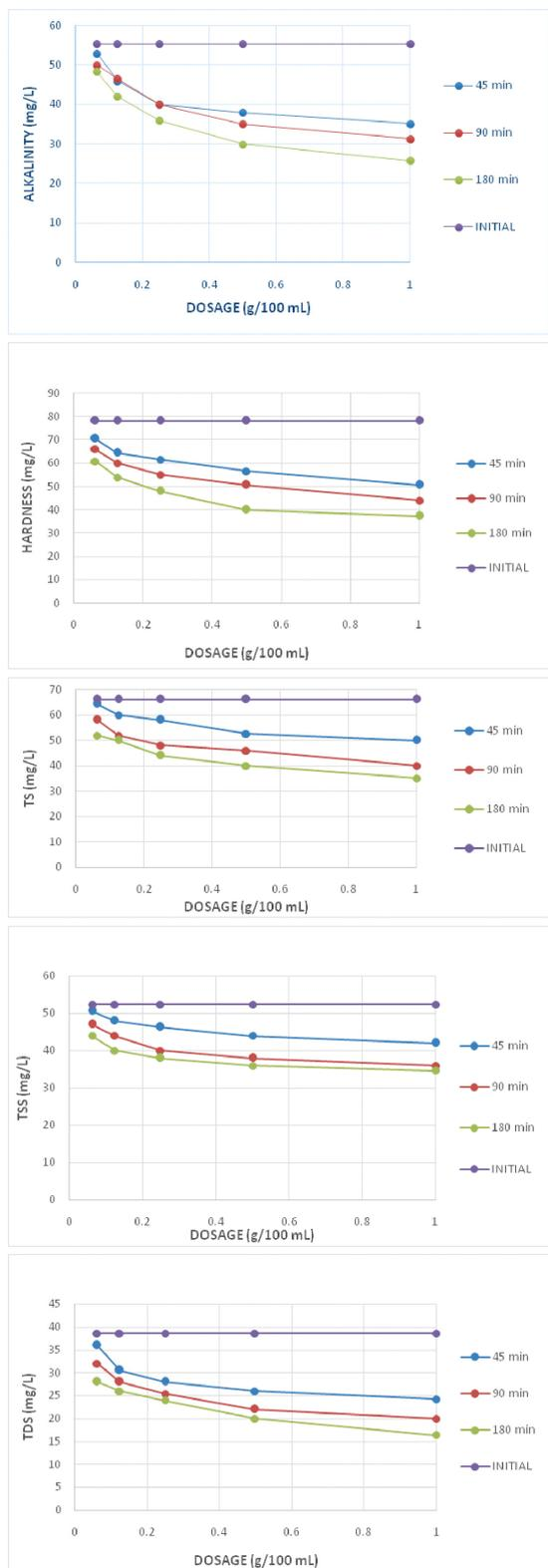
Fig. 2. Efficacy of fish scale adsorbent in the treatment of various water quality parameters of seafood processing industry effluent
