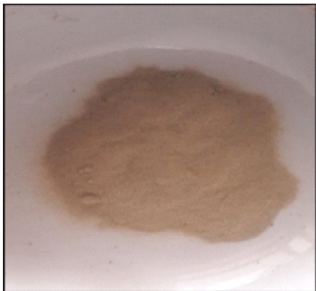
Fig. 1. Prepared fish scale adsorbent
