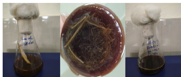
Fig. 1. a). Control raw feather b). Partially degraded raw feather by FMKB1 and FMKB2 within one month c). Completely dissolved raw feather by FMKB1 and FMKB2 within 45 days
